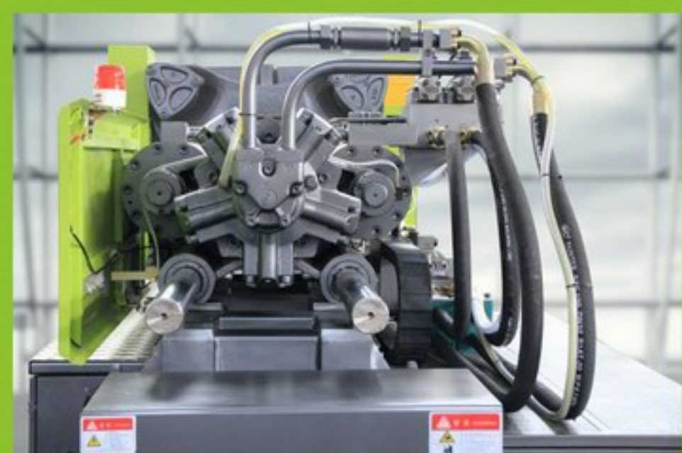
低速大扭矩液压马达驱动螺杆 Screw is driven by low speed & big-torque hydraulic motor
