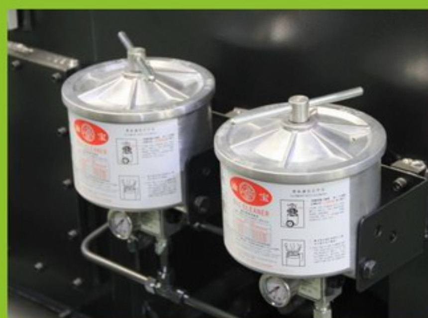
高精度回油过滤器全流量过滤油路 High-precision oil filter and full-flow by-pass oil filter
