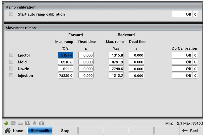
Fig.4-120: Mask "Automatic ramp calibration"
