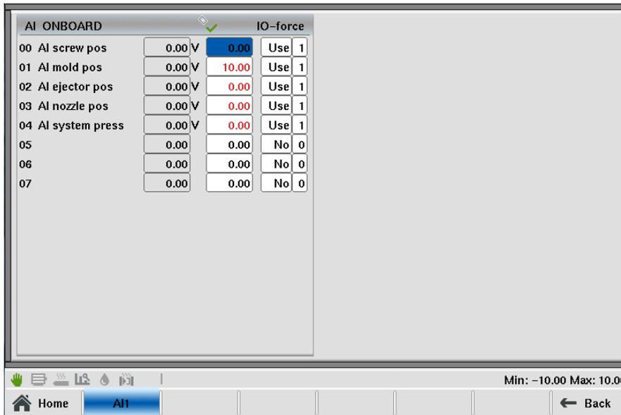
Fig.4-73: Mask 'IO Monitor analog Inputs'
